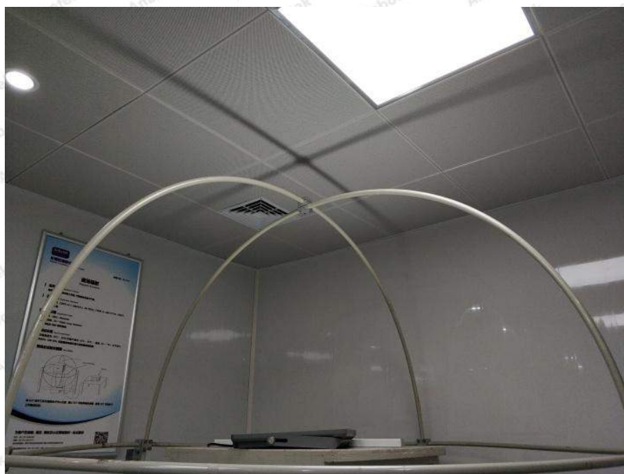
Photo of Magnetic Radiated Emission Test
