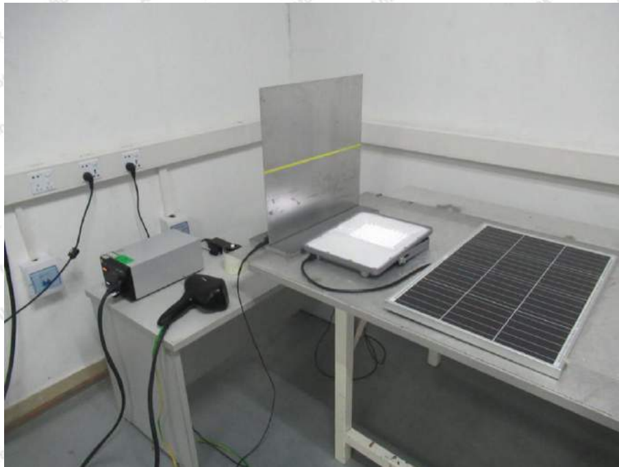
Photo of Electrostatic Discharge Immunity Test
